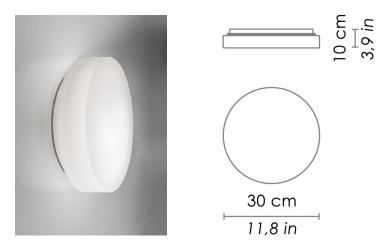
Wall-ceiling lamps with diffuser in mouth-blown, satin-finish opal triplex glass; chlorine-resistant, anti-UV, neutral translucent polycarbonate frame. Twist-lock coupling system for the glass component. The product is suitable for indoor use only. The Drum collection is IP44.
